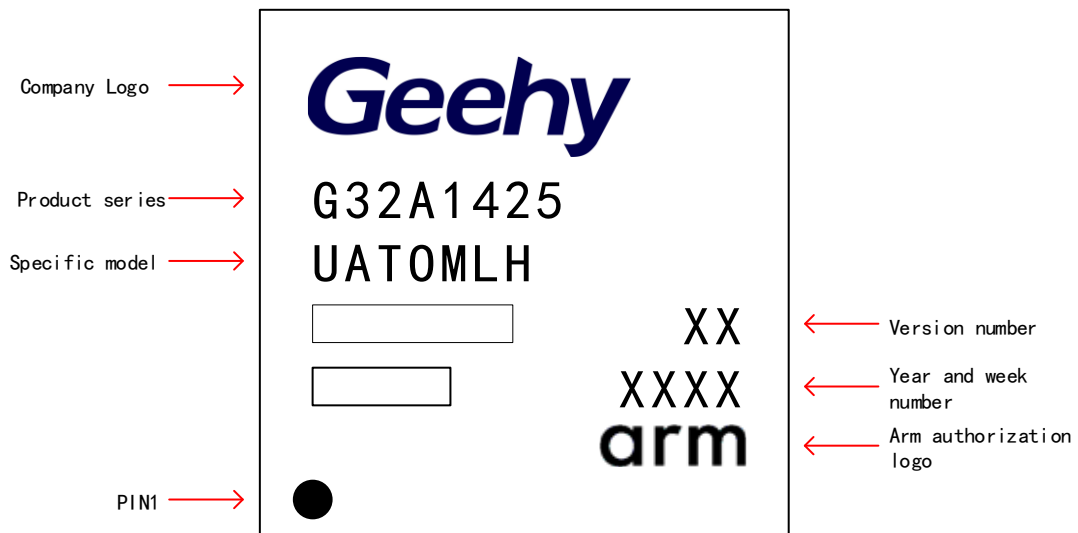
Figure 29 LQFP64 - 64 Pins, 10 x 10mm Diagram
